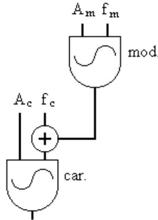
Figure 2-4. The oscillator configuration for the simple frequency modulation of a sine tone, where  $A_m$  = the modulator's amplitude,  $f_m$  = the modulator's frequency,  $A_c$  = the carrier's amplitude, and  $f_c$  = the carrier's frequency.
