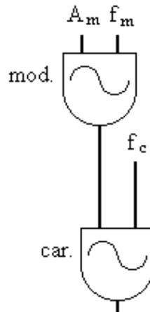
Figure 2-2. The oscillator configuration for the simple ring modulation of a sine tone, where  $A_m$  = the modulator's amplitude,  $f_m$  = the modulator's frequency, and  $f_c$  = the carrier's frequency.
