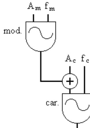
Figure 2-1. The oscillator configuration for the simple amplitude modulation of a sine tone, where  $A_m$  = the modulator's amplitude,  $f_m$  = the modulator's frequency,  $A_c$  = the carrier's amplitude, and  $f_c$  = the carrier's frequency.
